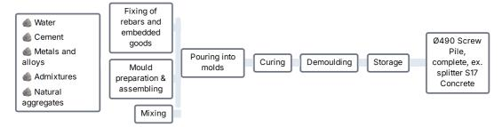
Centrum Prefabricated Screw Pille is particularly suitable as a pile foundation element in cohesive soil types with shear strengths up to 300-400 kN/m2 and in non-cohesive soils with CPT cone penetration test qc values up to 15-20 MPa.
